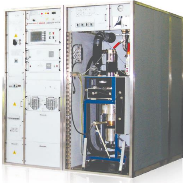
New CERN 801.6 MHz, 60 kW CW IOT TX. 9 units operational at CERN.
