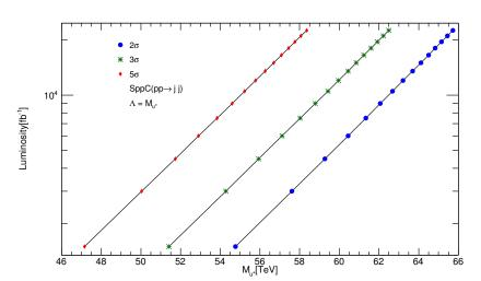
We scanned all luminosity ranges with respect to  $u^*$  mass which are planned to be achieved at SppC with  $\Lambda = M_{"}$  for 1500-22500  $fb^{-1}$  in 15 years.
