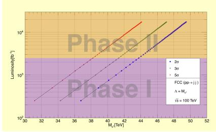
We scanned all luminosity ranges with respect to  $u^*$  mass which are planned to be achieved at FCC with  $\Lambda = M_{u^*}$  for Phase I (250-2500 fb<sup>-1</sup>) in 10 years and Phase II (2500-17500 fb<sup>-1</sup>) in 15 years.
