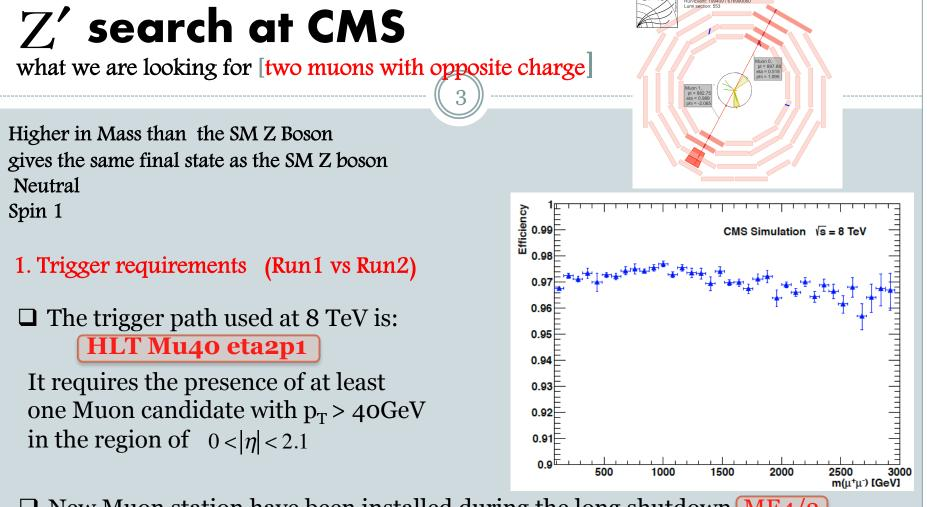
□ New Muon station have been installed during the long shutdown ME4/2 which covers the region  $2.1 < |\eta| < 2.4$
