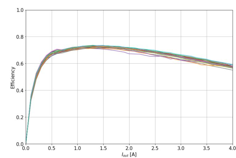
The efficiency of the DCDC converter is around 70% at the expected 2A load current.
