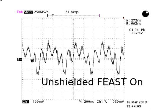
Shield box performance can be tested by measuring the noise on a coil placed below the Powerboard (above).
