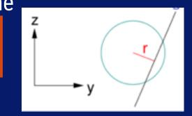
$b_{\pm}=\pm\sqrt{1+ar{m}^2}\cdot r-(ar{m}z_t-y_t)$  Each MDT chamber is composed of two multilayers (ML). For each ML we fill an histogram of bt, hits belonging to maxima in the histograms are selected and used for the segment fitting.
