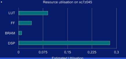
The implement algorithm is **fast and lightweight**. The resource utilisation on the FPGA for a single segment finder block is less than one third of the available resources. It is therefore possible to reconstruct muons in a trigger sector with a single Zynq 7045 chip. The algorithm runs at 240 MHz with a processing latency of only 245 ns, leaving more than enough time to transfer the data to the CPU and to perform the pT computation.
