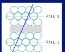
The trajectory of a high-pT muon in the yz plane can be approximate to a straight line within a single MDT chamber. y = mz + b
