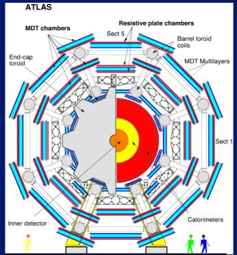
The upgraded L0 Muon Trigger of the ATLAS [0] detector will be divided into two subsystems. The first makes use of Resistive Plate Chambers (RPC) and Thin Gap Chambers (TGC), which have excellent time resolution (~ns), to identify possible high-pT muon candidates compatible with the considered pp bunch crossing (BX).
