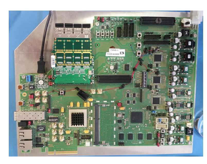
Over the last years the Bologna Division of I.N.F.N. and the Physics Department of the University of Bologna have collaborated to the ATLAS Pixel Detector upgrade designing the ROD (Read-Out-Driver) board for the off-detector read-out system. The ROD boards are mainly devoted to data formatting as well as detector configuration, calibration and triggering; about 100 RODs have been installed and are now in operation.
