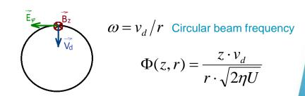
In case of <u>non</u> azimuthally uniform beam there could be an angular component of the electric field causing beam to tilt by  $\Phi$ .
