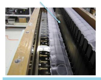
AD – Mechanical Support Electrostatic Septa Wire Failures (100 μm) after 20 years in beam 120 kV, 14 mm
