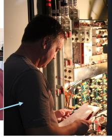
Computer and FPGA control of large power supplies, 50 ppm regulation of 1200 A, learning systems
