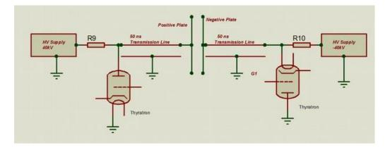
The shorted line method, with magnetic pulse sharpening, is an attractive solution and has been demonstrated at J-Parc.
