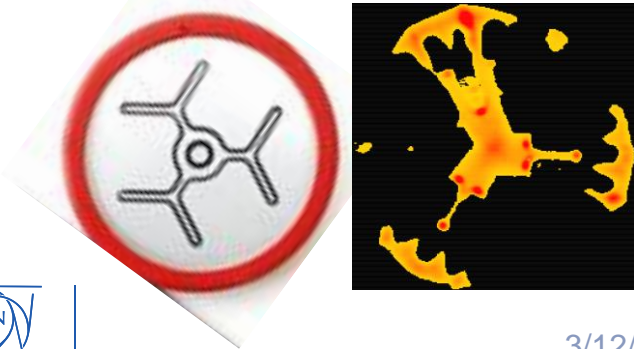
Mapping of the area illuminated above the threshold intensity. 49uJ light pulse.
