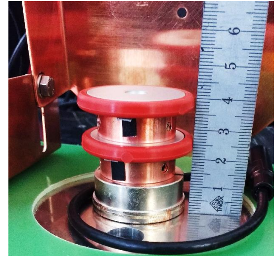
Two stacked wafers placed in the low inductance clamp
