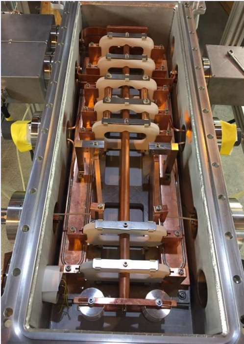
Prototype kicker in vacuum chamber
