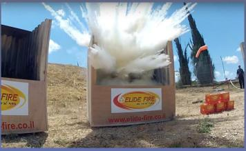
WHEN THE FLAME DETECTOR IS ACTIVATED, IT LAUNCHES CO2 PACKAGES
