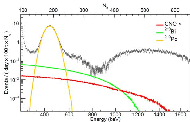
**CNO, <sup>210</sup>Bi and <sup>210</sup>Po energy spectral shapes and the Borexino detected events (black)**
