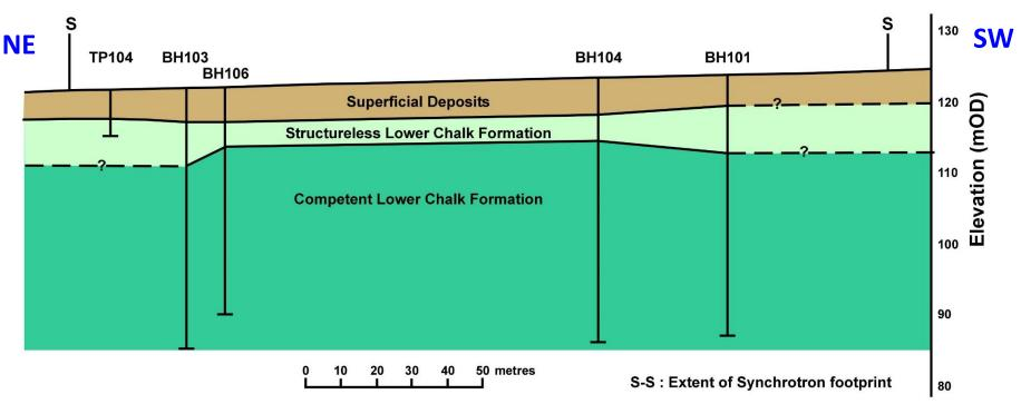
NE-SW Geological cross-section interpreted through the centre of the Synchrotron (based on Norwest Holst Engineering Ltd., 2001)
