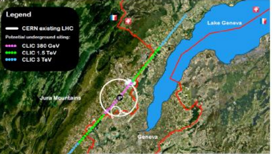
Compact Linear Collider (CLIC) e + e + , \sqrt{s} = 380 GeV, 1.5 TeV, 3 TeV Length: 11 km, 29 km, 50 km
