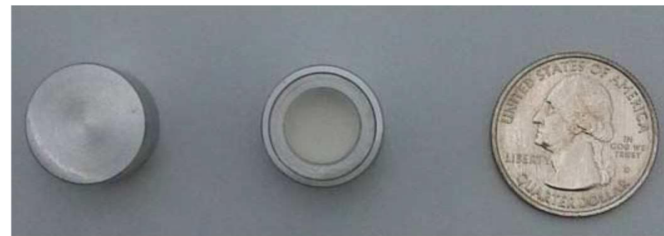
Fig. 2. LaBr_3:Ce scintillation crystal pair contained by aluminium boxes of glass bottom windows.
