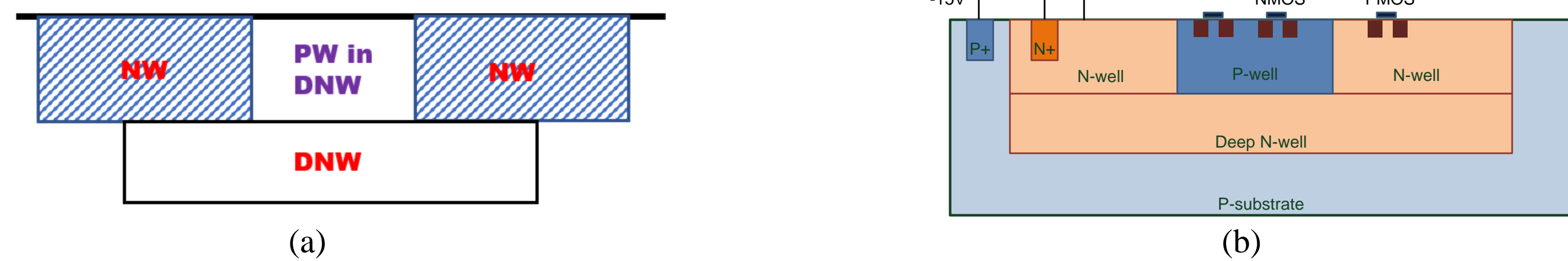
Fig. 1. Diagram of the sensor characteristics(a) and in pixel circuit(b)
