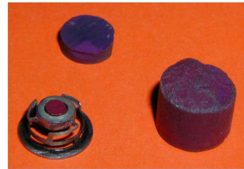
cathodes damaged by sputtering
