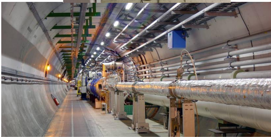
“Combined” sector Both beams circulates in the same beam pipe
