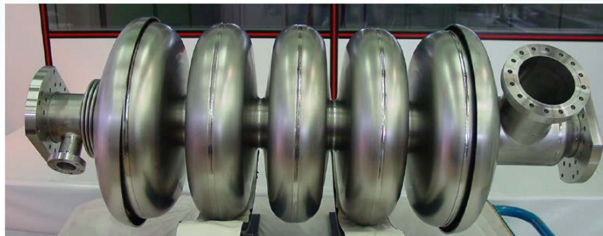
\beta = 0.65 , 704 MHz elliptical cavity
