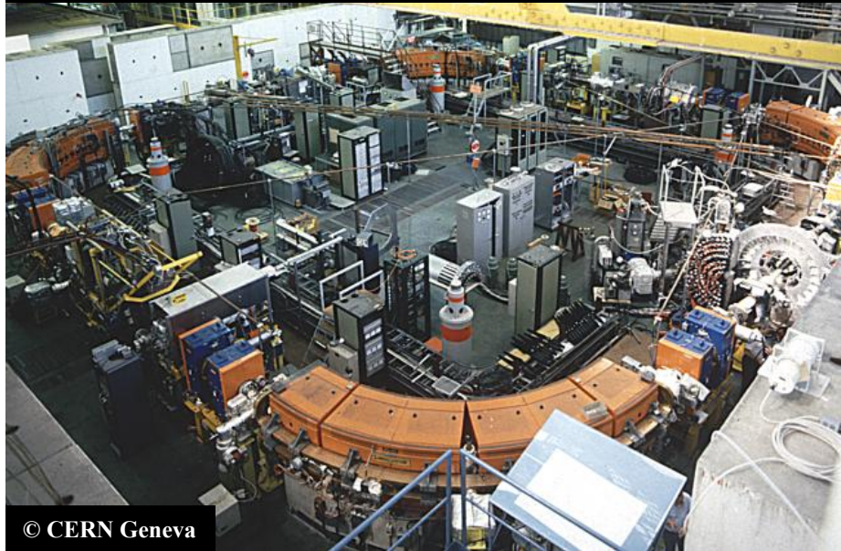
LEAR (CERN) Low Energy Antiproton Ring
