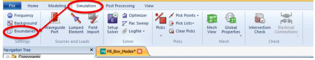
Particularly, in order to find the TM modes let's impose the condition of zero tangential electric field at the wall, as shown below:
