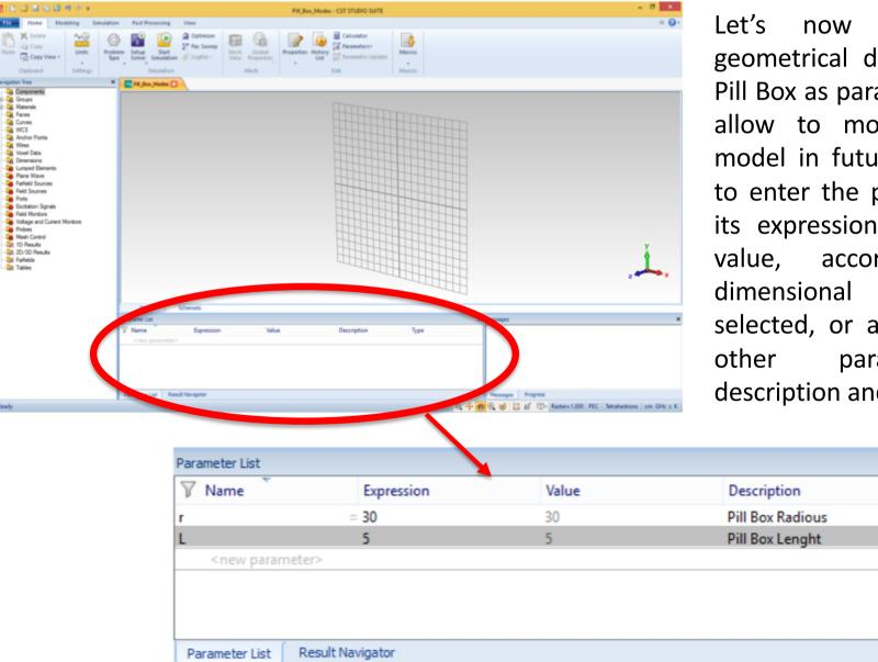
Let's now introduce the geometrical dimension of the Pill Box as parameters. This will allow to modify the entire model in future. It is possible to enter the parameter name, its expression (it could be a value, according to the dimensional units previously selected, or a combination of other parameters), its description and its type.
