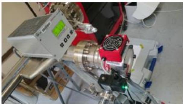
Figure 3: Turbomolecular pump system → 10^{-6} mbar
