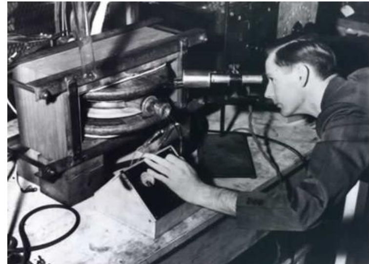
Donald Kerst with the first betatron, built at University of Illinois in 1940
