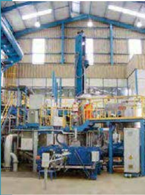
Fig. 4.4: A re-melting furnace for the production of pure titanium with 2 x 600 kW e-beam power (courtesy of ALD Vacuum Technologies).
