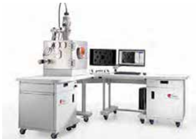
Fig. 4.8: A desk-top e-beam laboratory machine for welding and structuring with a magnified backscattered electron-image.
