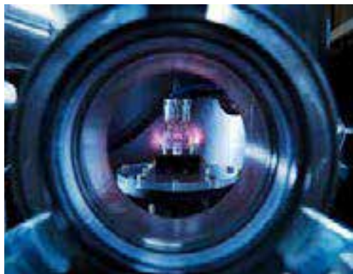
Fig. 2.10: A plasma cell developed as part of an EU-supported project, EuPRAXIA, to study plasma accelerators for applications (credit: Heiner Müller-Elsner/DESY).
