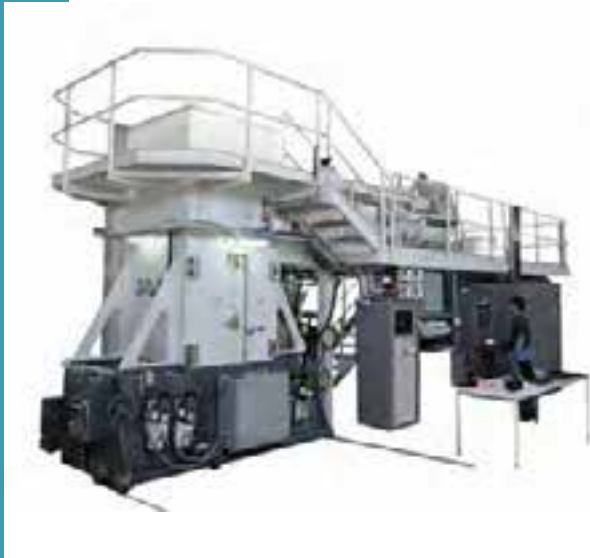
Fig 4.16: IBA's Easy-e-Beam™ Integrated system for cross-linking small wires for the automotive market.
