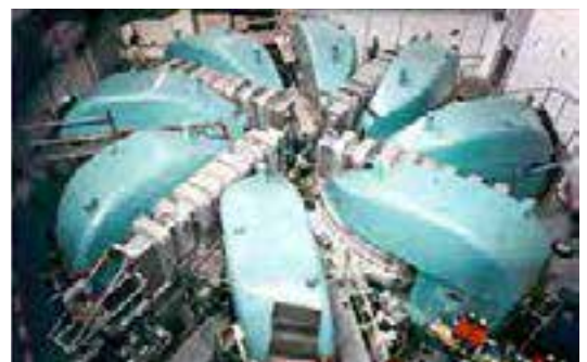
Fig. 2.5: The PSI 600-MeV cyclotron. This is currently the highest-energy cyclotron in operation and the highest-power accelerator in the world.
