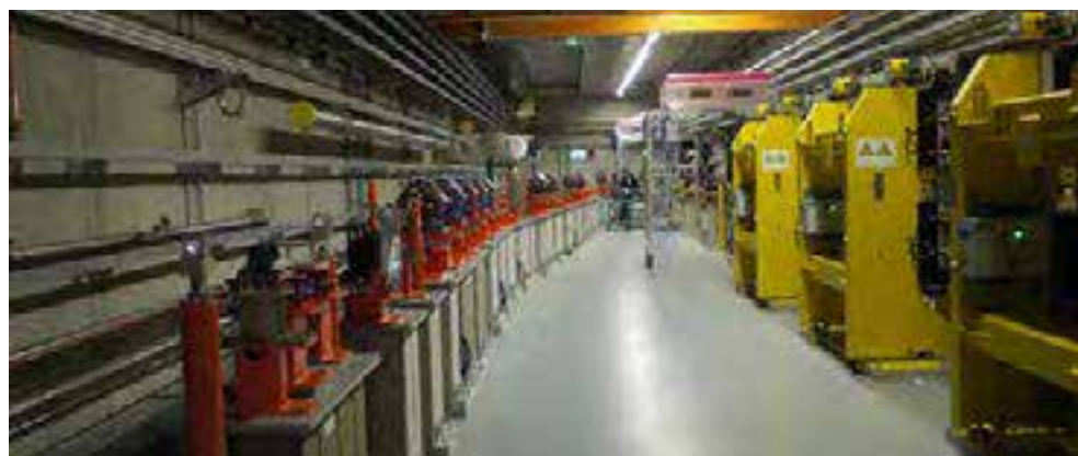
Fig. 7.10: The FLASH accelerator project at DESY, which is testing plasma acceleration; a compact plasma accelerator could feed an electron beam to an FEL or synchrotron source.
