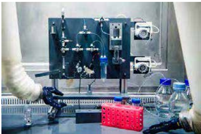
Fig. 3.16: A semi-automated production module at PSI for the purification of radionuclides involving the use of ion-exchange chromatography.
