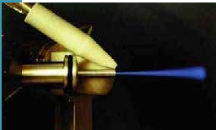
Fig. 4.18: A 3-MeV proton beam extracted into air.
