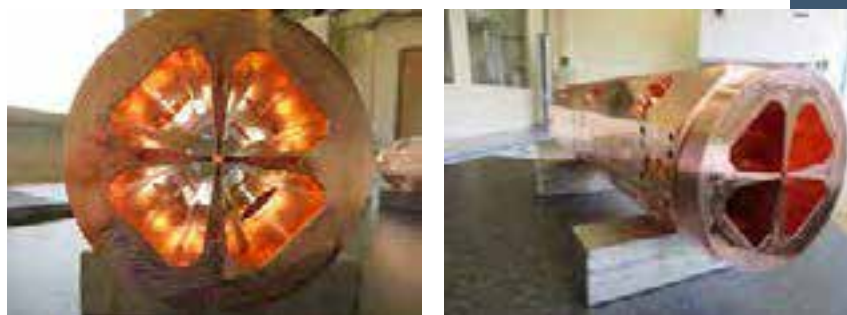
Fig. 8.9: Compact RFQs are being developed for proton accelerators suitable for many applications including medical therapy, nuclear transmutation and neutron spallation (credit: S. Hills).
