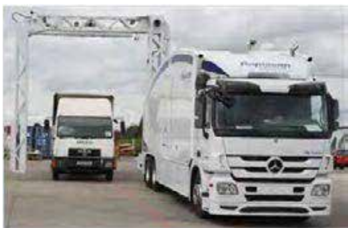
Fig. 6.2: Rapiscan's mobile high-energy X-ray system for inspecting cargos at border crossings.
