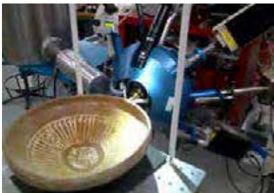
Fig. 4.22: PIXE and PIGE at AGLAE were used to determine the elemental composition of an ancient bowl from a shipwreck (credit AGLAE/ J. Burlot).
