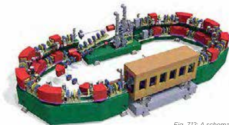
Fig. 7.12: A schematic of a compact light source to be commercialised by Advanced Accelerator Technologies (Switzerland).
