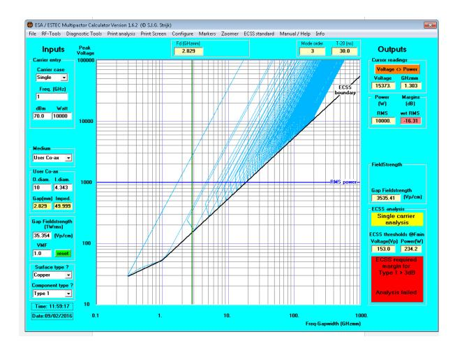
You see that with 100 watt travelling wave power you are still safe, but 100 Watt traveling wave power are just 1 Watt input power on a resonator with a Q of 100
