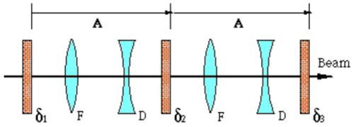
where A is the transfer matrix of the FODO cell without the skew lenses. Let matrix A have the phase advance  $\mu_0$  in both planes and express the matrix at the mid-point between F and D ( $\alpha_m$ ,  $\beta_m$ ).
