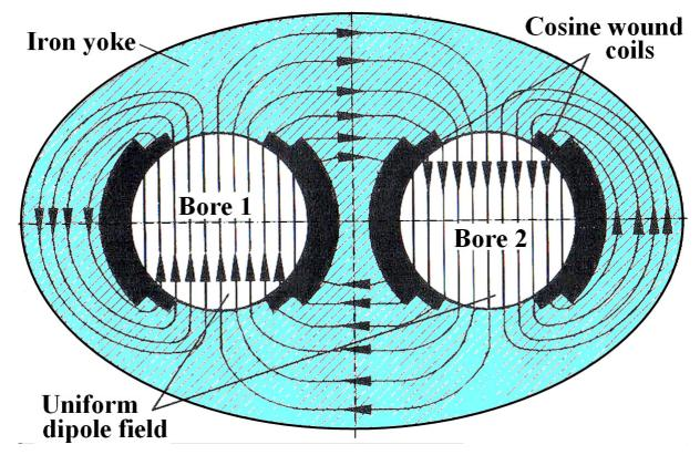
The twin-bore design is used in the LHC. This choice was driven mainly by the lack of space in the already existing LEP tunnel.
