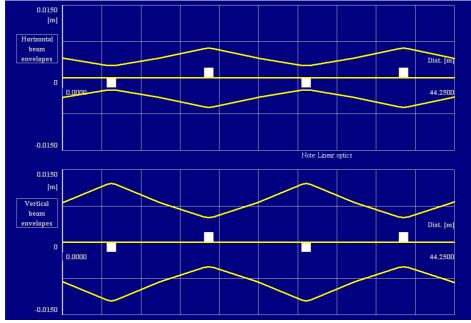
Inverter with skew quads powered.
