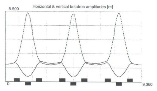
The sigma matrices can be used to track the beam sizes through the rotator. Terms m<sub>11</sub> and m<sub>33</sub> give the beam width and height on the orthogonal p-q planes (see last lecture).
