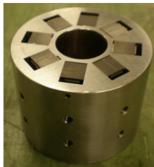
LINAC4 DTL PMQ, < 1 kg
