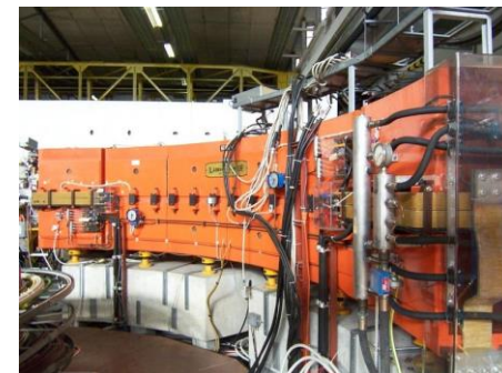
LEIR main dipole, 60 tons
