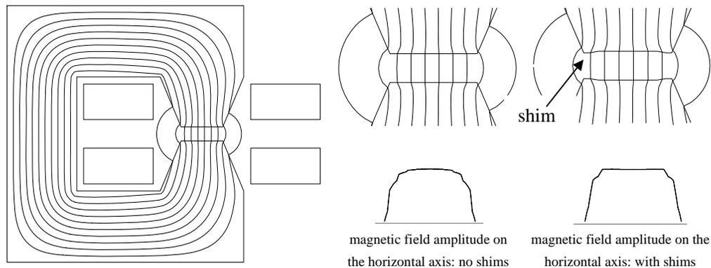
C-dipole with pole shims. The shims extend the good field region
