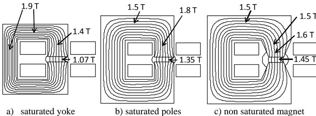
C-dipole magnetic circuit, of physical vertical aperture  $l_{air}=10$  mm, supplied with  $N_{tot}I=120\ 000A$ .
