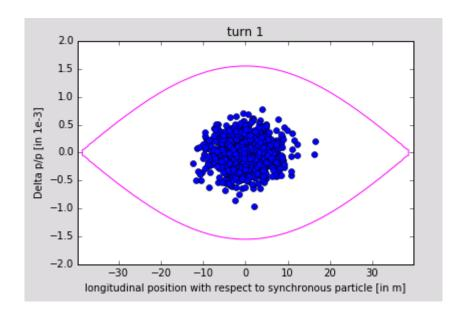
It is the same case as case A with a change of variables. the shape of the bucket is symmetric and therefore not accelerating. the synchronous phase is 0, therefore we are below transition.
