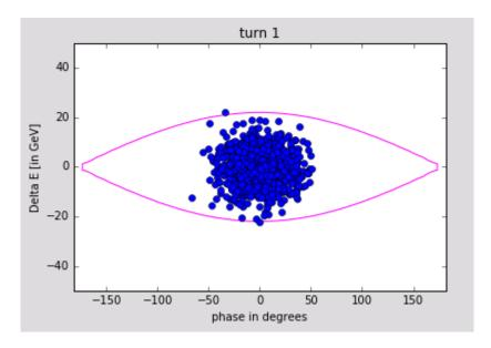
Phase acceptance =2 pi → we are in a stationary bucket (i.e. no acceleration)
