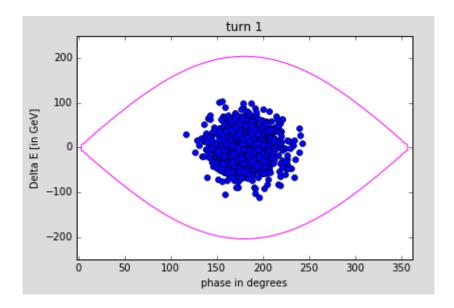
Phase acceptance =2 pi → we are in a stationary bucket (i.e. no acceleration)
