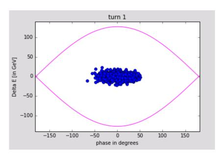
Phase acceptance =2 pi  $\rightarrow$  we are in a stationary bucket (i.e. no acceleration)
