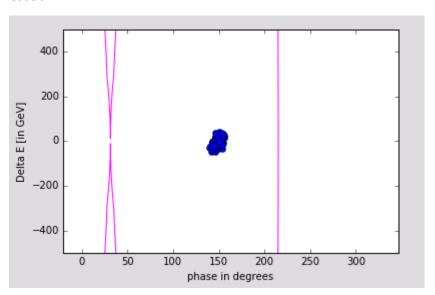
Phase acceptance < 2 pi → we are in non stationary bucket (i.e. acceleration or deceleration)
