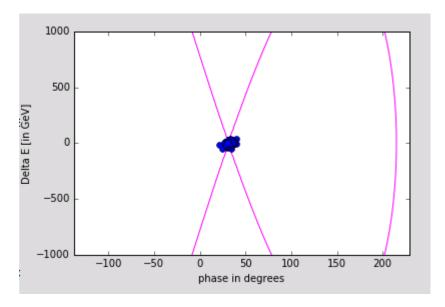
Phase acceptance < 2 pi → we are in non stationary bucket (i.e. acceleration or deceleration)
