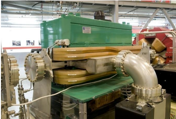
Sextupole magnets to focus off-energy electrons (mainly)
