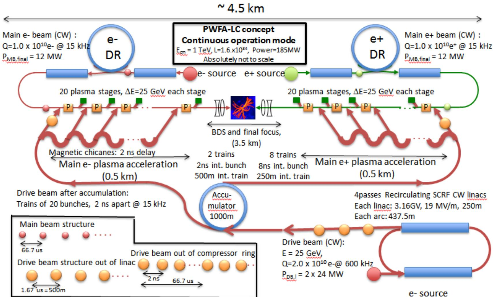
Concept for PWFA-LC layout for 1 TeV. Based on earlier work from 2009 by Raubenheimer et al. E. Adli et al., "A beam driven Plasma Wake-Field Linear Collider", CSS2013 and arXiv:1308.1145
