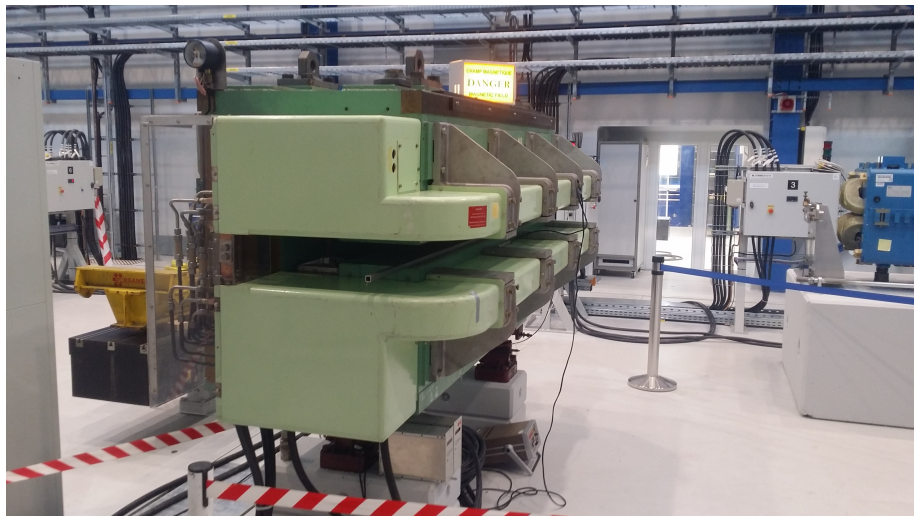
Figure: Magnet that has been characterised during the 2nd part of the practical
