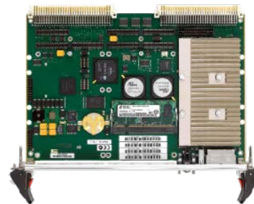
VME Card: Eurocard size VMEbus interface
