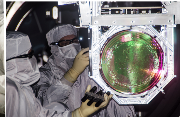
Inspecting reaction mass with the ESD. Protected with First Contact
