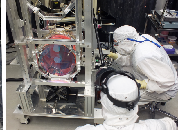
Welding silica fibres to test masses.
