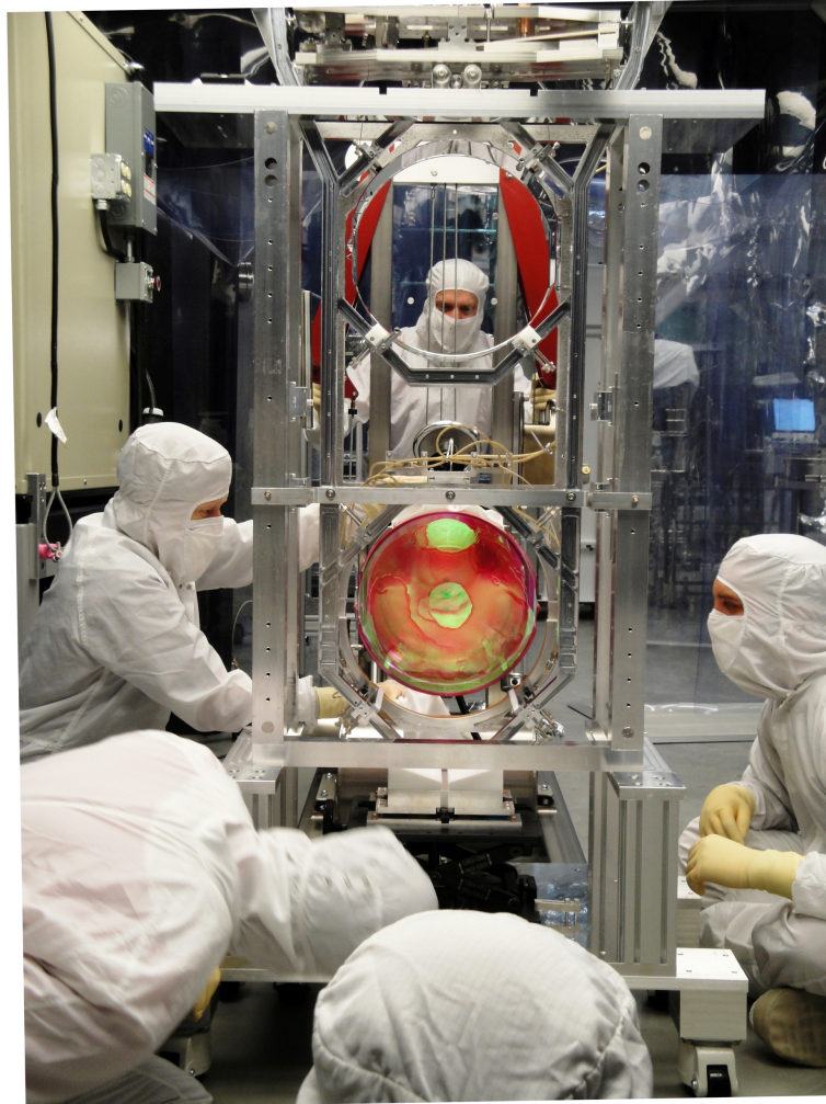
Inspecting last stage of the pendulum suspension. Monolithic of fused silica.
