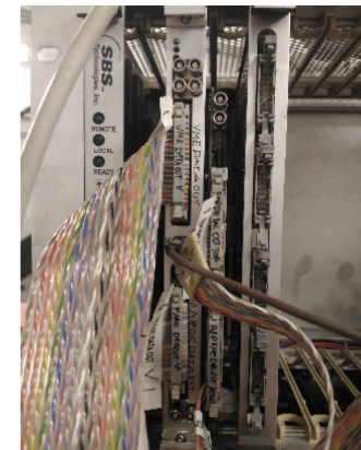
Figure 5: New VME board compact communication board, cabled to the tagging modules via flat cables, and the VME side of the SBS (Bit3) controller, installed in the BTF experimental area.
