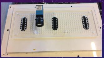
Camera set up in previous AIDA FP7 "Glycol" cold box to avoid fogging of optics from LN2 boil off. Aligned and focussed on optical target shown bottom left
