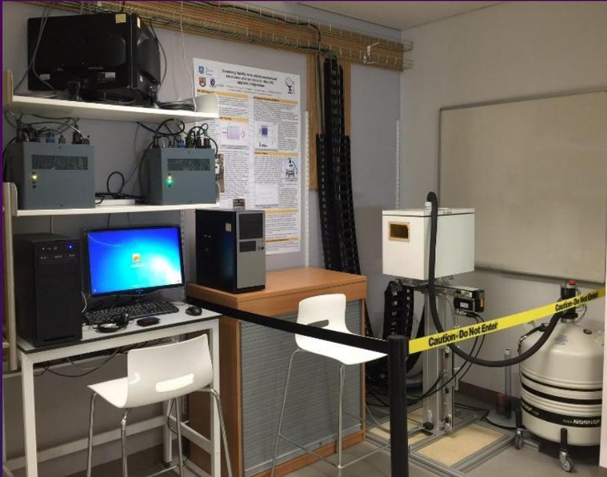
To test and implement upgrades to the scanning system and software, a second scanning system and LN2 cooling unit is undergoing installation in [Sheffield Robotics](#). Sited in the 300m<sup>2</sup> Robotics Foundry in the new purpose built 7 story, 5355m<sup>2</sup> Pam Liversidge Building for “Interdisciplinary Research”.
