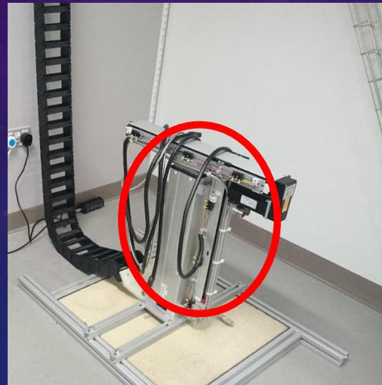
The assembly of the new custom made lifting pillar is now completed with a modified pillar housing to accept the new motor made in Sheffield.
