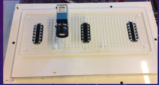
Camera set up in previous AIDA FP7 "Glycol" cold box to avoid fogging of optics from LN2 boil off. Aligned and focussed on optical target shown bottom left
