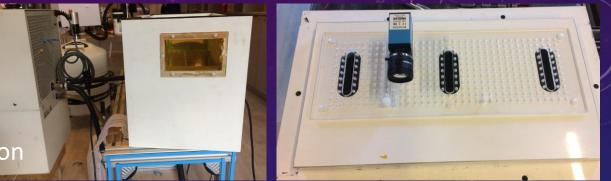
Camera set up in previous AIDA FP7 "Glycol" cold box to avoid fogging of optics from LN2 boil off. Aligned and focussed on optical target shown bottom left
