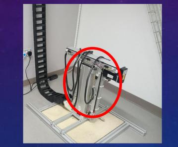
The assembly of the new custom made lifting pillar is now completed with a modified pillar housing to accept the new motor made in Sheffield.
