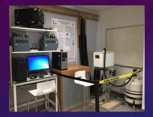
To test and implement upgrades to the scanning system and software, a second scanning system and LN2 cooling unit is undergoing installation in <u>Sheffield</u> <u>Robotics</u>. Sited in the 300m<sup>2</sup> Robotics Foundry in the new purpose built 7 story, 5355m<sup>2</sup> Pam Liversidge Building for "Interdisciplinary Research".
