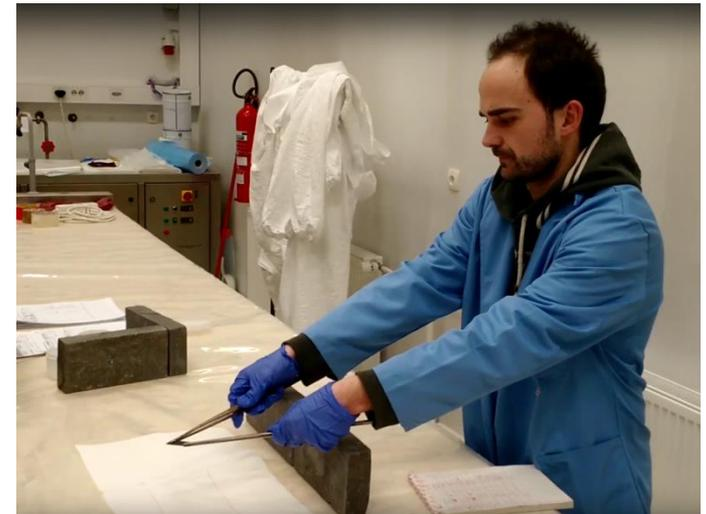
*Stress tests on the samples irradiated at JSI*
