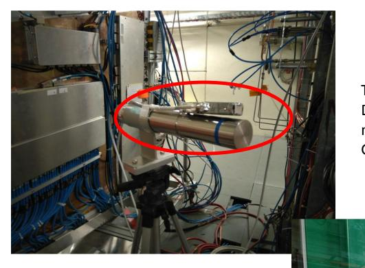
Test position of the RADMON Integrated Dose Monitor + Berthold GM dose-rate monitor Upstream and Downstream at Gif++
