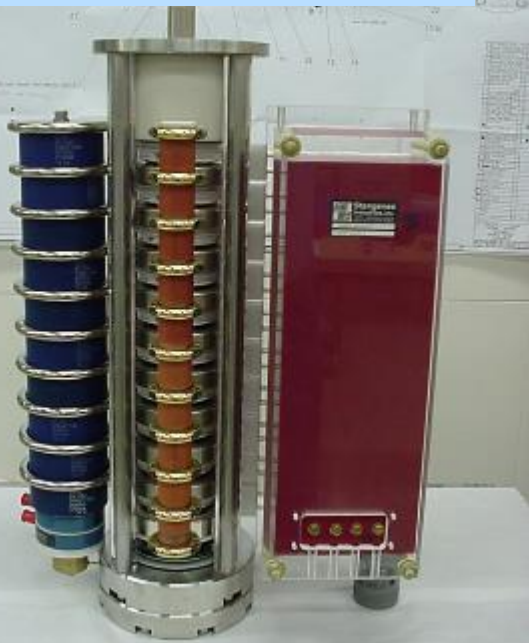
FHCT stack with trigger transformer
