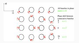
With four possible phase shifts between the four bunches, above transition, n=1 is UNSTABLE.
