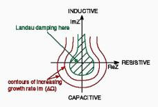
The line defining zero growth rate leads us to a handy approximation for the stability limit of unbunched beams, the 'Keil-Schnell Stability Criterion':
