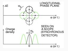
The single bunch in 'dipole' or 'rigid bunch' mode rotates in longitudinal phase plane with  $\omega_s$ , the phase  $\phi$  and energy  $\Delta E$  also vary with  $\omega_s$ .
