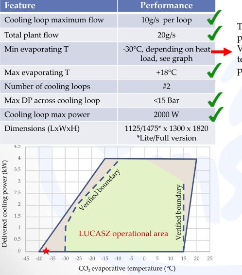
The minimum temperature performance is not (yet) met in Lucasz-V1a (some modifications needed). 1<sup>st</sup> tests with V1b showed better performance (-38.5'C, no load)
