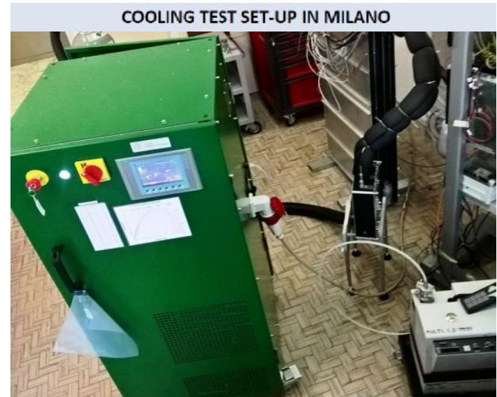
CO 2 TRACI V.3 COOLING SYSTEM
