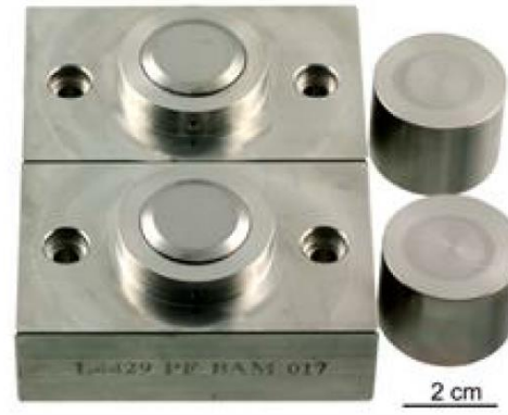
Fig. 2. Samples: left: Ti6Al4V pads; right: steel 316LN cylinders
