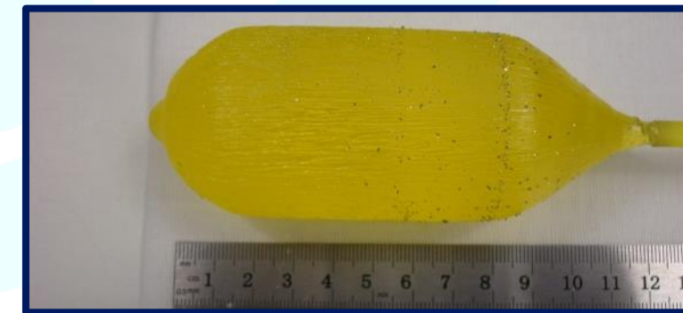
As-grown GGAG:Ce Crystal 50 mm in dia.
