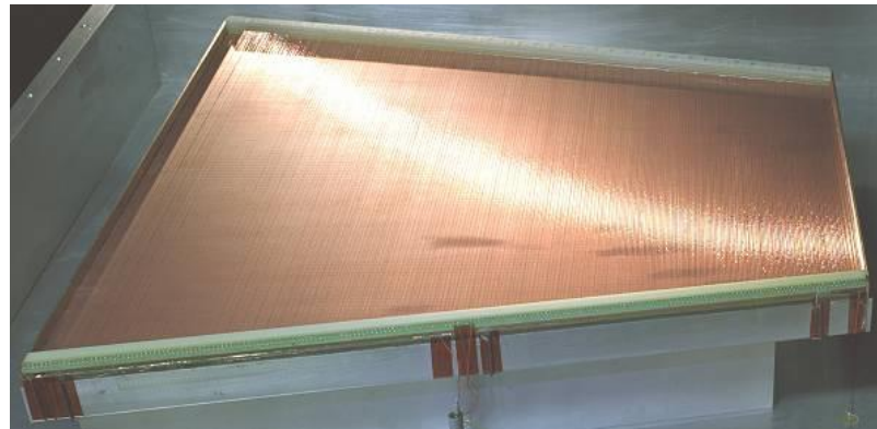
Wire chamber: 40 \mu m
