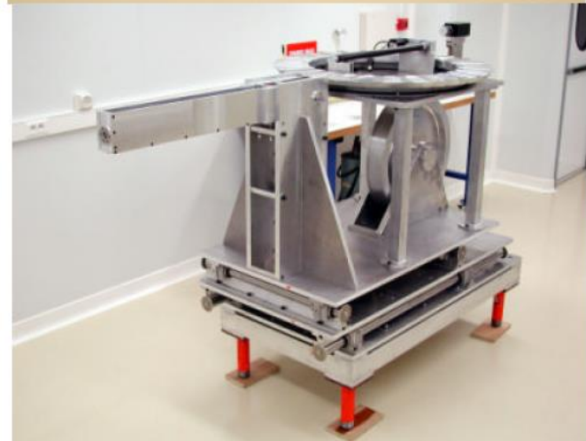
"Carousel" brick dispensing and storage system
