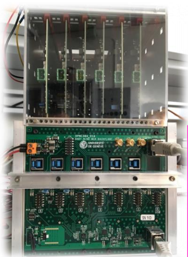
BACK: USB SYNC/CLOCK in MCB out (emul.) MCB in (emul.) 24V Leds/Address Prog.
