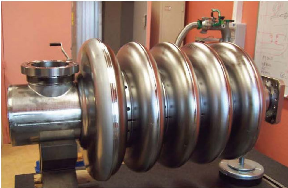
Elliptical 5 cell bulk Niobium cavities (e.g.: \beta=0.47 )
