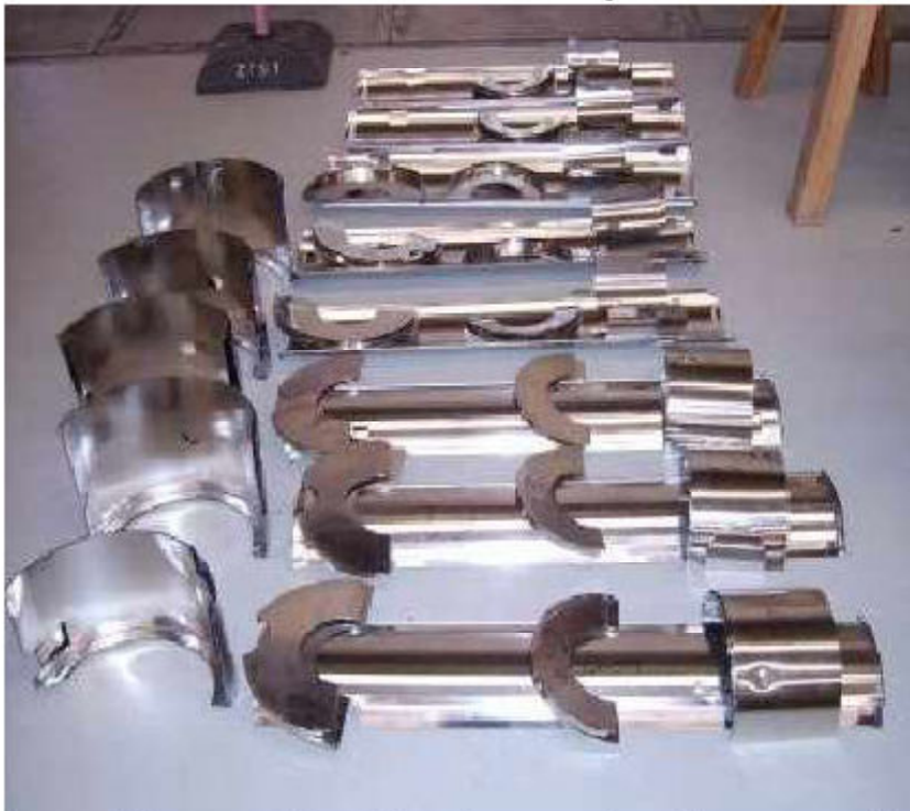
Single parts of magnetic shield and assembly of magnetic shielding
