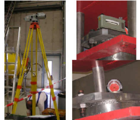
Figure 36: Optical leveler (left), water level and Taylor Hobson ball (right)
