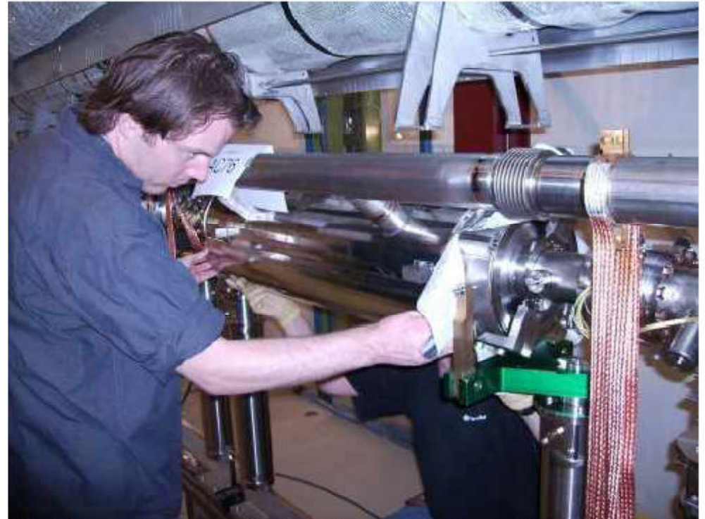
Single parts of magnetic shield and assembly of magnetic shielding
